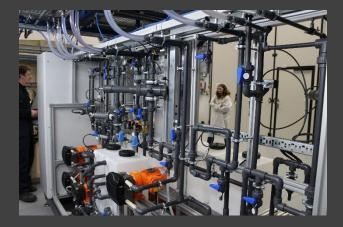
Near Real Scale Test and Control Water Treatment Works
